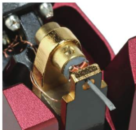
Visible just behind the cantilever hinge are two of the four micro-coils that sit on an iron yoke. Behind lie parts of the magnetic circuit. At front is a pole plate.
