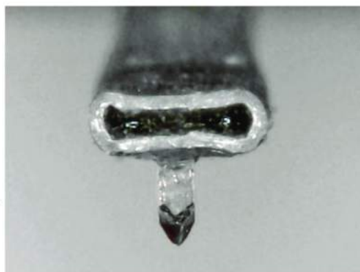
The dark tip appearance suggests it can be profiled by laser, rather than grind wheel, the original way to profile a Shibata – purposed for 1970s CD4 discs.
